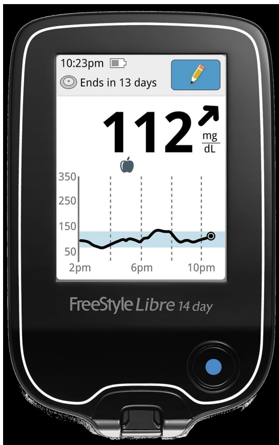
Figure 1. A representative image of the FreeStyle Libre 1 sensor and reader. The sensor is worn on the upper arm and continuously measures interstitial glucose levels, which can be scanned using the handheld reader to obtain real-time glucose data.
